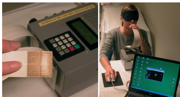
FIGURE 1. THE TONGUE DISPLAY UNIT (TDU) AND ITS COMPONENTS.
